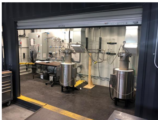
Figure 2. Titanium Sponge Production System – Laboratory Setup
