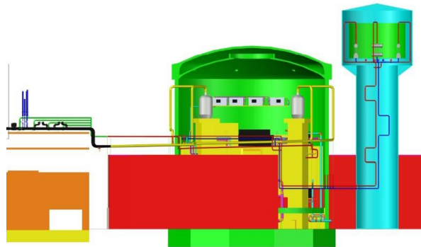
Figure 1. Passive Safety System for CANDU 6 Cernavoda Unit 2 NPP
