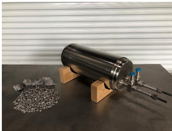
Figure 1. High Purity Titanium Sponge and Immobilized Tritium Container – Lethal Service
